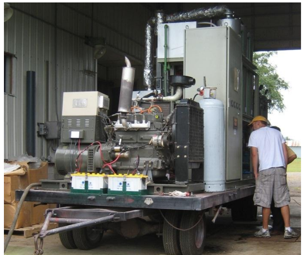
Figure 3. Pilot scale mobile MAP system developed through previous LCCMR and other projects; with incorporation of microwave absorbents, it becomes fMAP, a superior fast thermochemical conversion process.
