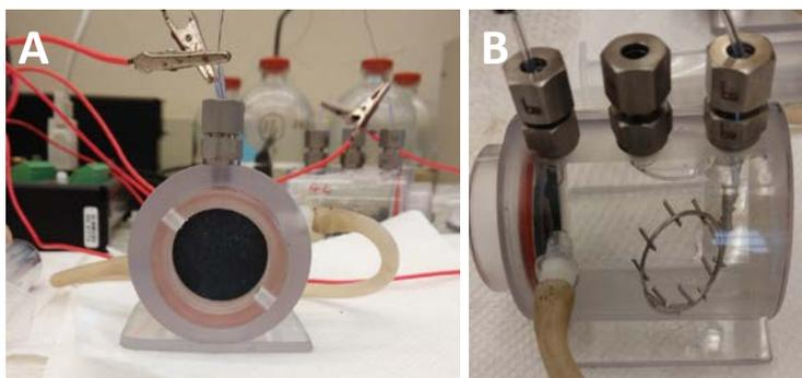
Figure 3. Air-cathode reactors. A, end-view; and B, top-view.
