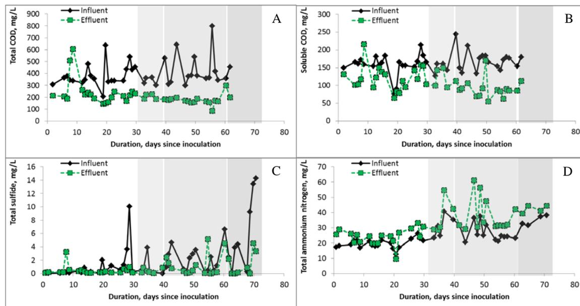
Figure 38. Evolution of the influent and effluent total COD (A), soluble COD (B), total sulfide (C), total ammonium nitrogen (D) content.
