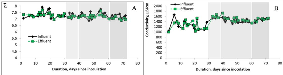
Figure 35. Evolution of the influent and effluent pH (A) and conductivity (B).
