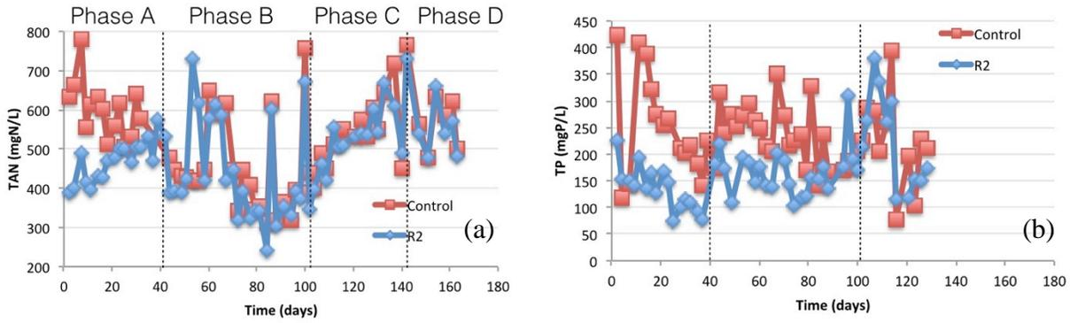
**Figure 24.** (a) Total ammonium nitrogen (TAN) concentration in the effluent of both reactors 'Control' reactor and CSTR-MEC reactor (R2). (b) Total phosphorous in the effluent of both reactors 'Control' reactor and CSTR-MEC reactor (R2).
