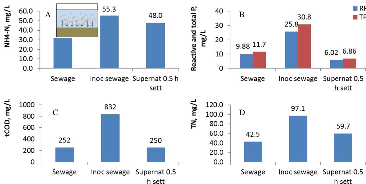
Figure 11. Initial separation of nutrients due to the sedimentation of particulates.
