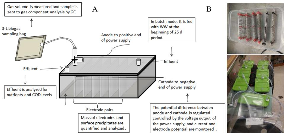
Figure 9. Illustration (A) and photos of simulated septic tanks (B).
