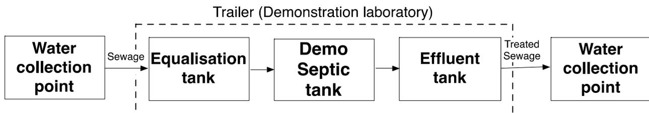
**Figure 29.** Process chart for the demonstration experiments.
