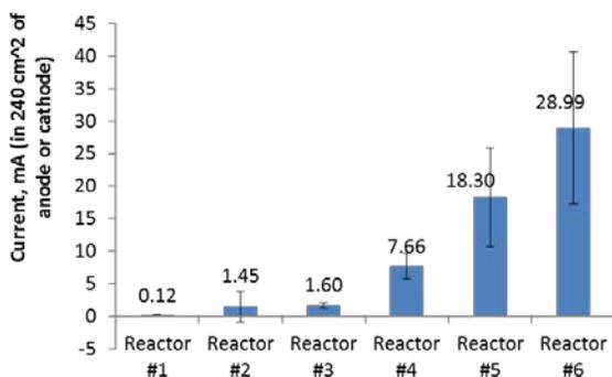
Figure 10. Current density in each voltage levels (0.25 V to 1.50 V with a 0.25 V increment).
