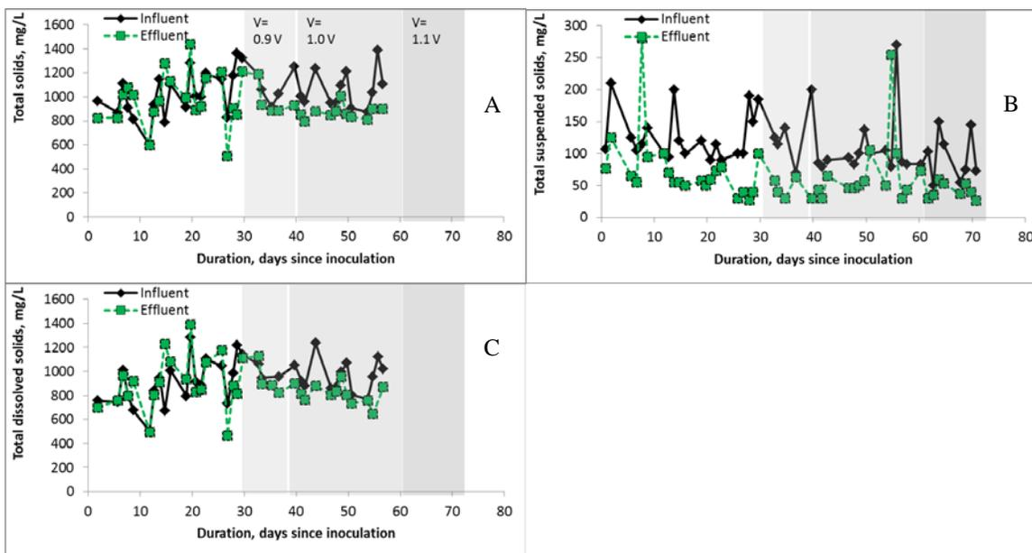
Figure 37. Evolution of the influent and effluent solids profiles: total solids (A), total suspended solids (B), and total dissolved solids (C).
