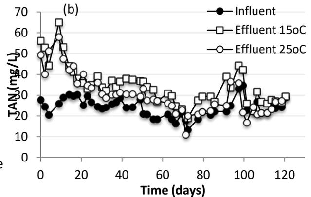
**Figure 31.** Evolution of the influent and effluent concentrations in the 20-liter lab-scale prototype reactors operated at 15 °C and 25 °C; (a) total solids and (b) total ammonium nitrogen, TAN.
