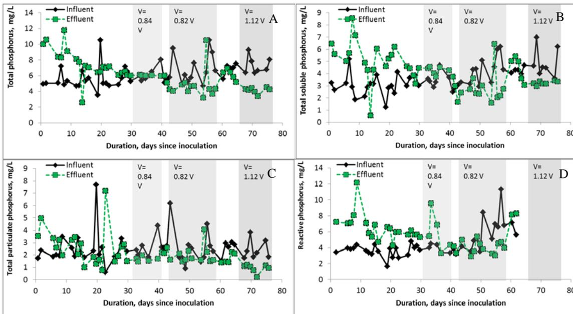
Figure 36. Evolution of the influent and effluent phosphorus profiles: total phosphorus (A), total soluble phosphorus (B), total particulate phosphorus (C), and reactive phosphorus (D).
