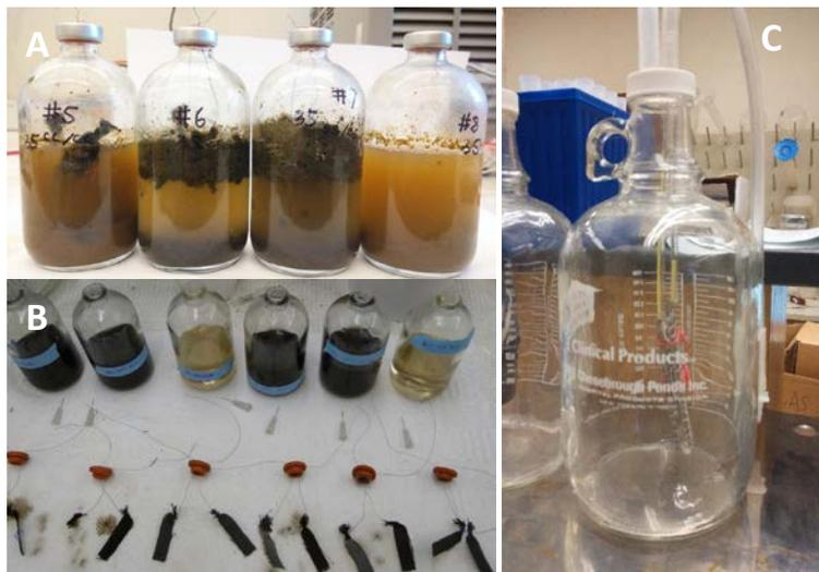
Figure 2. Serum bottle reactors. A and B, 150 mL reactors with media and electrode couples; and C, 1.5 L reactor vessels.
