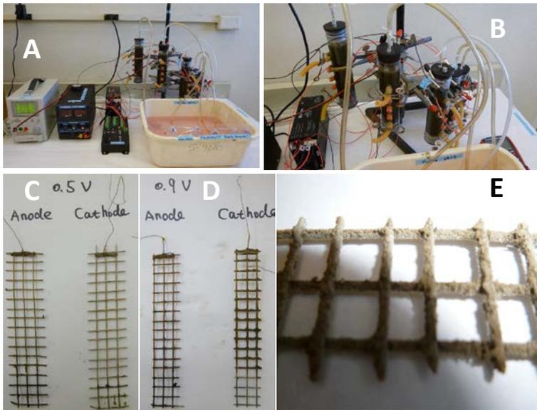
Figure 1. Up-flow column reactors. A and B, overview of the reactors and peripheries; and C, D, and E, electrodes after operations.
