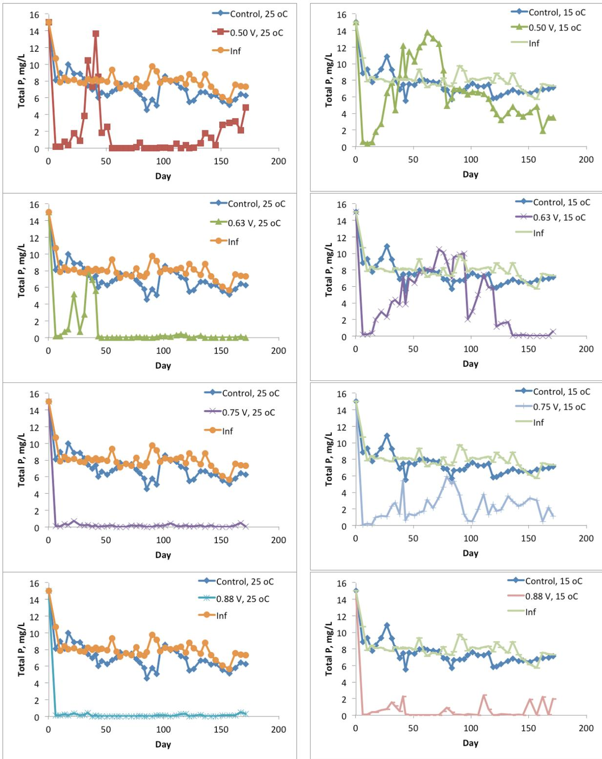
Figure 17. Total phosphorus in the influent and effluent of the reactors operated at different applied voltage and temperatures.
