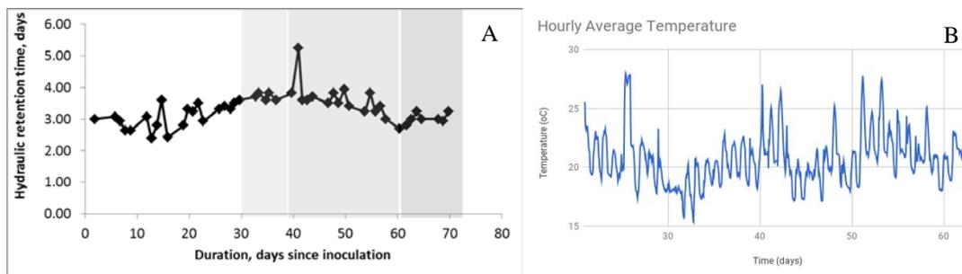
Figure 34. The hydraulic retention time (A) and experimental site room temperature (B).
