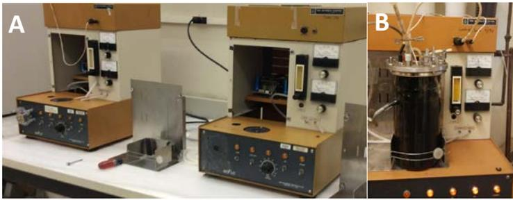
Figure 4. CSTR reactors prepared from fermenters. A, vessel holder and control systems; and B, CSTR in operation.
