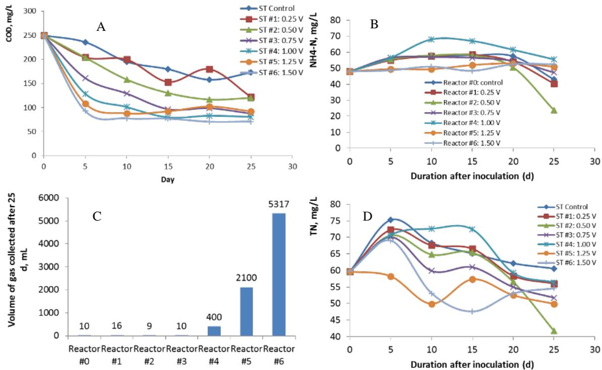
Figure 14. Nutrients profiles during operation and gas generation.
