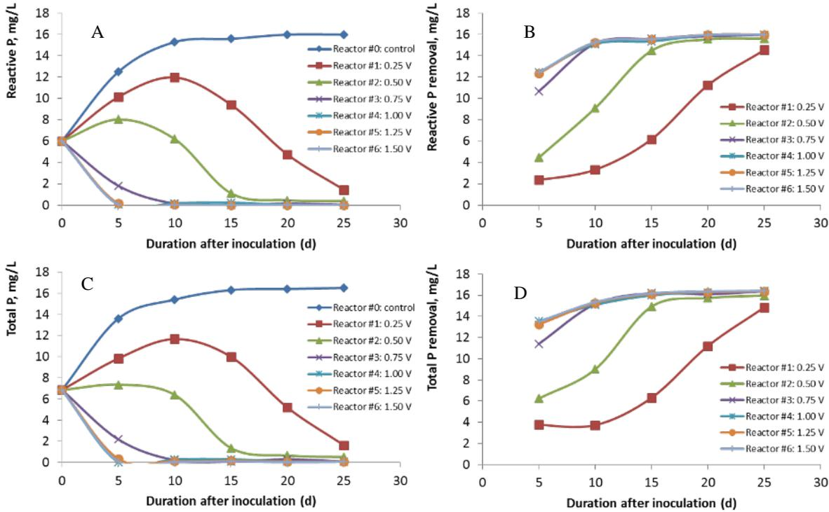
Figure 13. Phosphorus evolution during 25 days' operation of the reactors.
