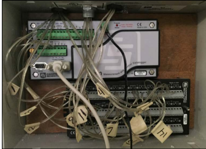
Figure 1: Campbell Scientific CR800 Data Logger with Campbell Scientific AM 16/32B Multiplexer.
