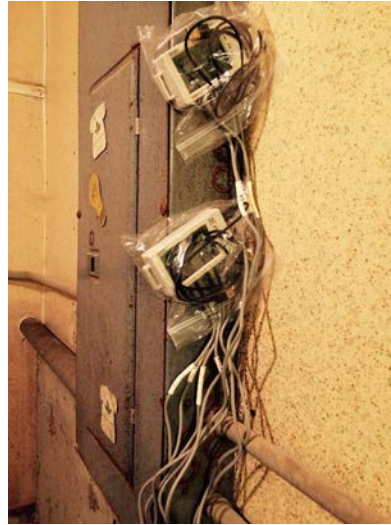
Figure 5. Data loggers attached to side of electric circuit breaker panel
