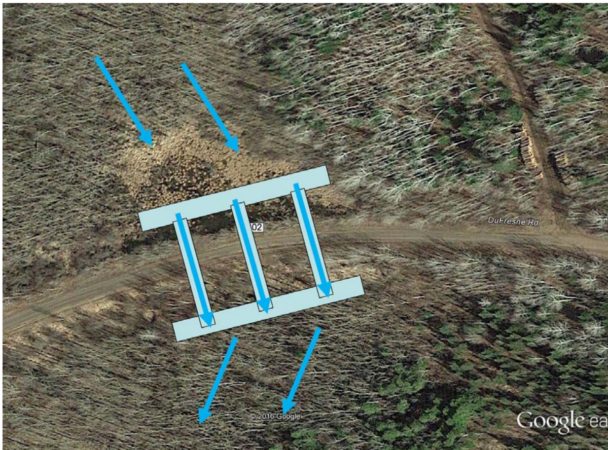
Figure 42. Modified H-culvert design used for Defense site. Blue arrows indicate water flow. Blue boxes represent buried rock trenches.
