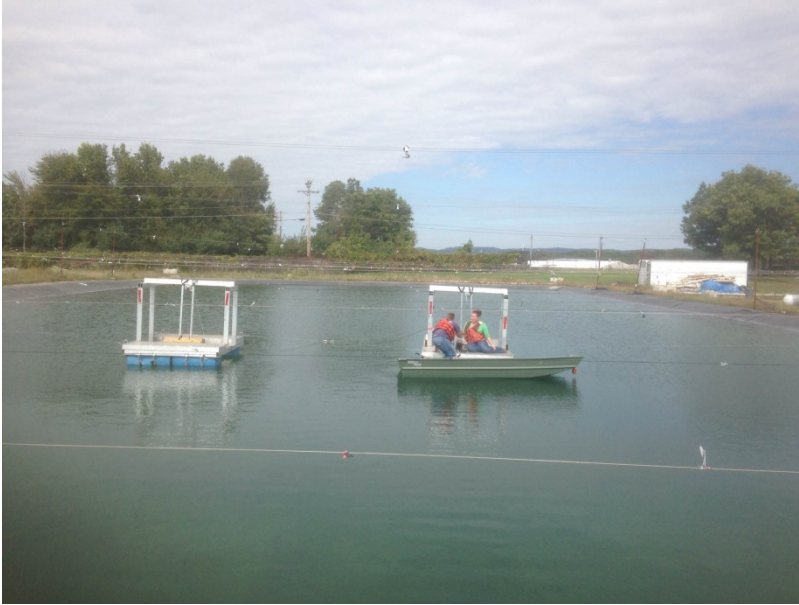
Figure 5. Position of the floating platforms that suspended the speakers in the 1/2 acre pond
