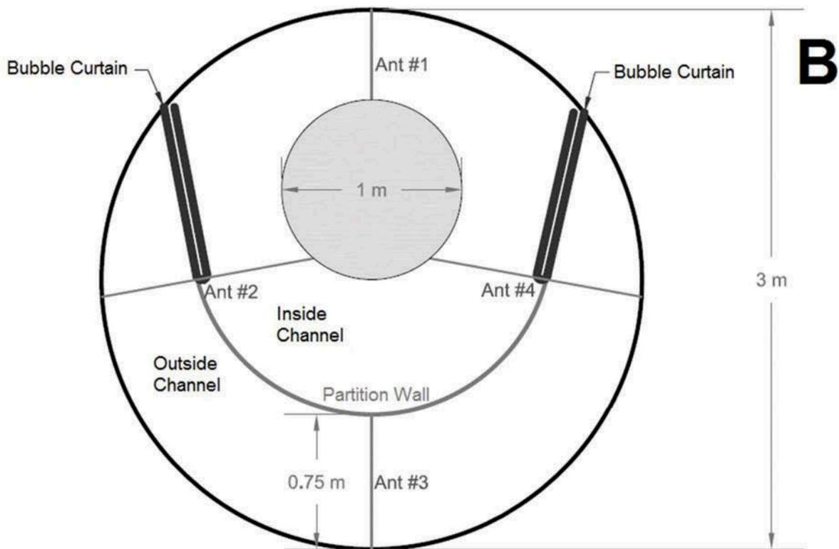
FIGURE 1. (A) Top view of the experimental bubble curtain tank. Bubble curtains (90 cm long white PVC pipes) are located at the end of the 50-cm-high partition wall. Water depth was 25 cm. (B) Overhead schematic of split-path circular channel showing position of bubble curtains and PIT antennas. Antenna number 3 was tuned and positioned to only detect movement through the outside channel.
