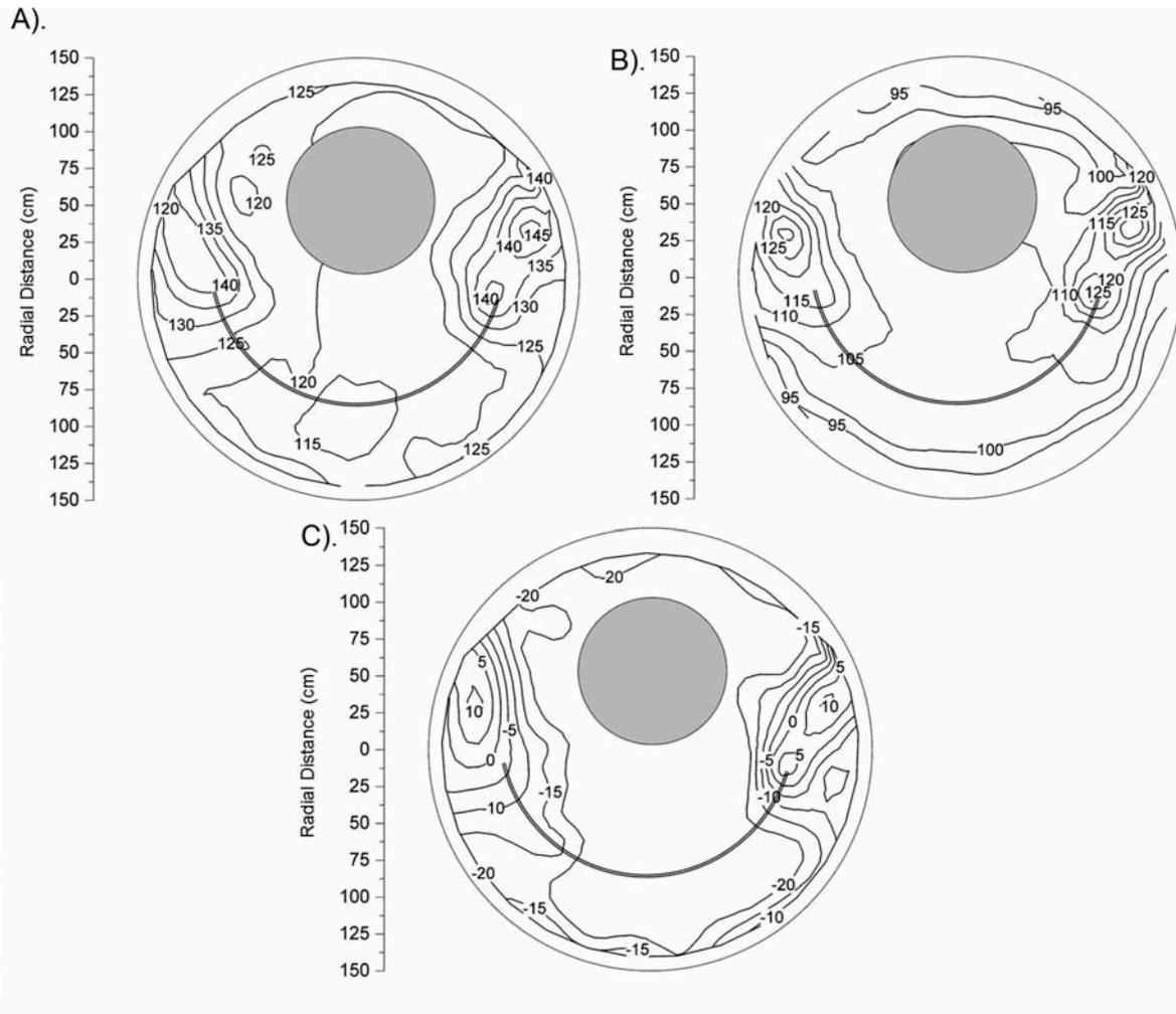
FIGURE 5. Plan view of the sound pressure field in decibels (ref  $1\mu\text{Pa}$ ) in the experimental tank at a depth of 12.5 cm at (A) 200 Hz, (B) 1,000 Hz, and (C) acoustic particle acceleration in dB (ref  $1\text{ cm/s}^2$ ). The bubble curtains extended tangentially from the ends of the partition wall (curved line). The background sound pressure level at 200 Hz and 1,000 Hz was 80 and 60 dB ref  $1\mu\text{Pa}$ , respectively.
