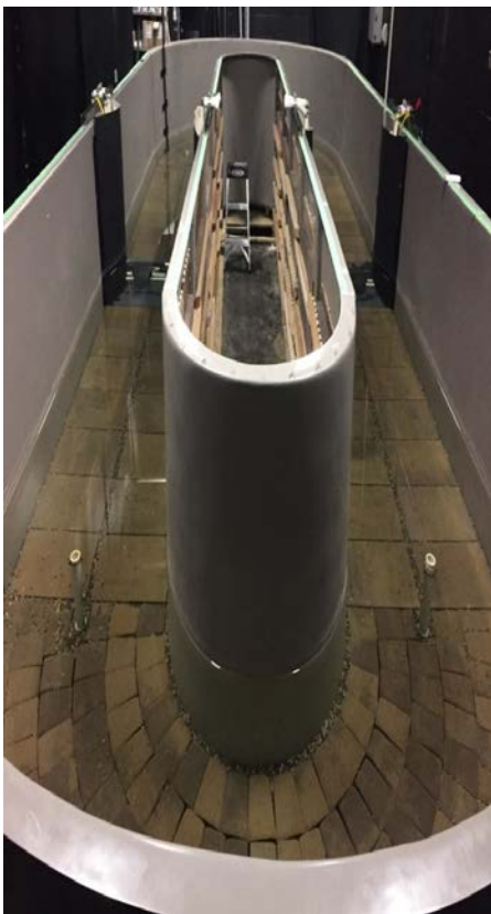
FIGURE 3-9. Custom built circular flume (26m long x 3m wide) used for laboratory behavioral tests examining the avoidance response of carps to different aversive stimuli.
