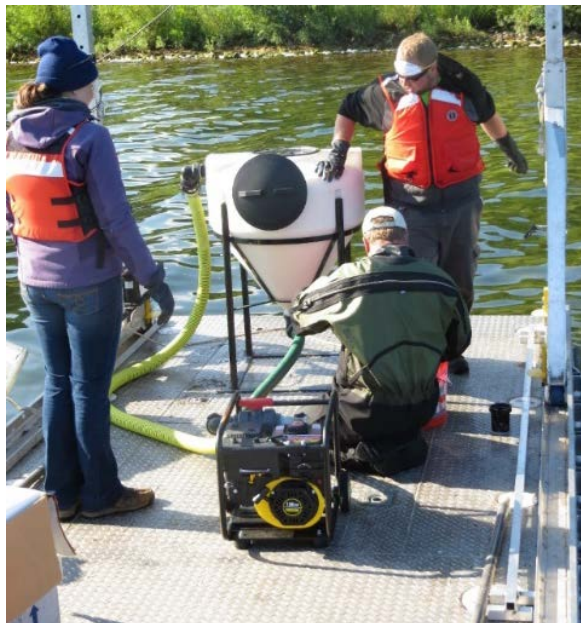
Figure 5. Zequanox suspension mixing system that was used to prepare the 5% (w/v) Zequanox suspensions for application to test enclosures in Robinson's Bay, Lake Minnetonka, MN.
