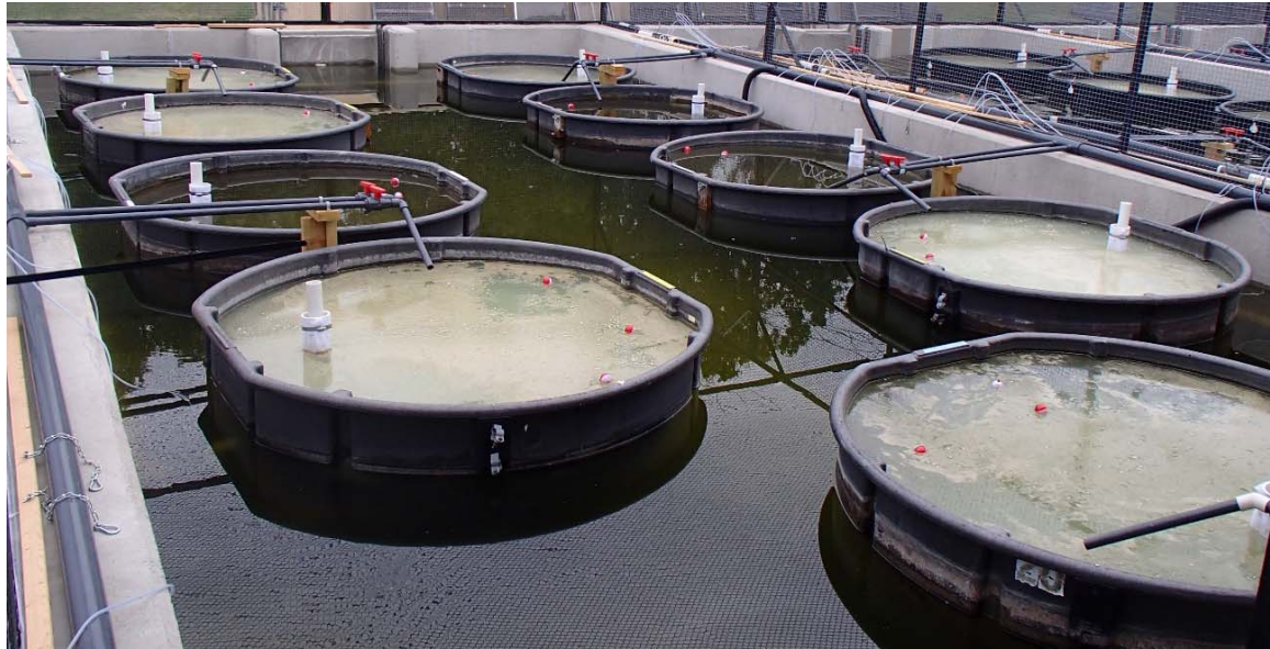
Figure 1. Mesocosm test system consisting of nine 1000-L tanks within each of two 0.004 ha concrete ponds. Water was supplied to test tanks from a 0.25 ha earthen pond. Concrete ponds were filled with water and covered with shade cloth to moderate diurnal temperature fluctuation.
