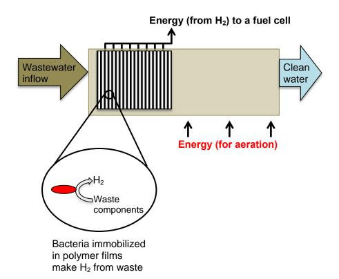
With the proposed technology, aeration requirements are reduced (saving energy) and energy (H<sub>2</sub>) is produced within specialized polymer films during an anaerobic (no aeration) phase of treatment
