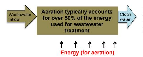
In traditional wastewater treatment, energy is used to aerate (and therefore treat) the wastewater
