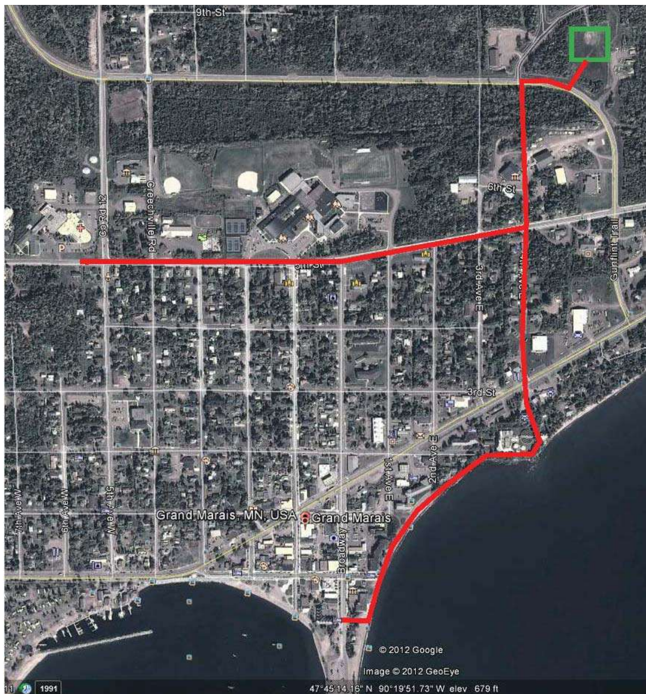
Figure 3. Preliminary Routing of Hybrid Scenario Distribution System
