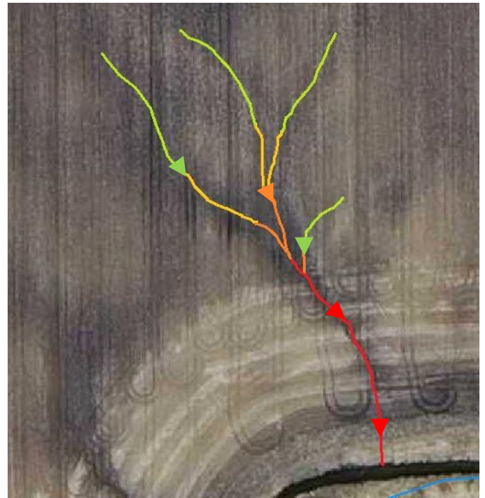
Figure 5. The above images depict how an SPI signature can be visualized as a flow path. The arrows represent flow direction
