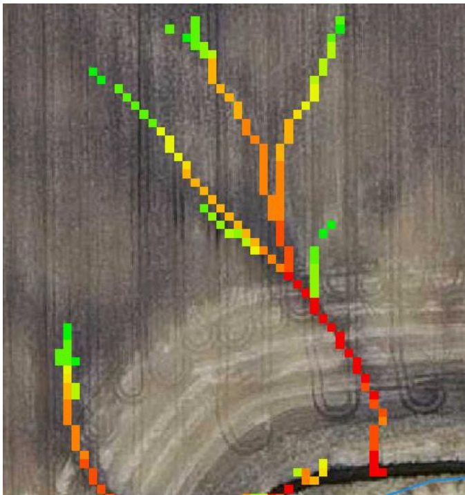
Figure 5. The above images depict how an SPI signature can be visualized as a flow path. The arrows represent flow direction
