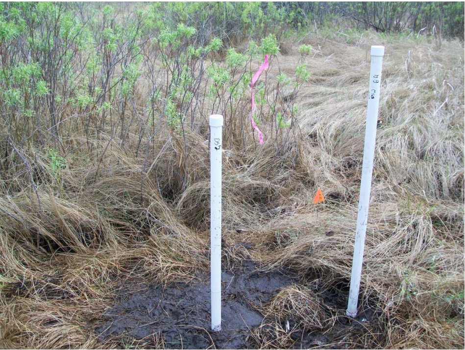
Piezometer DS2 and DS5 (deep piezometer)
