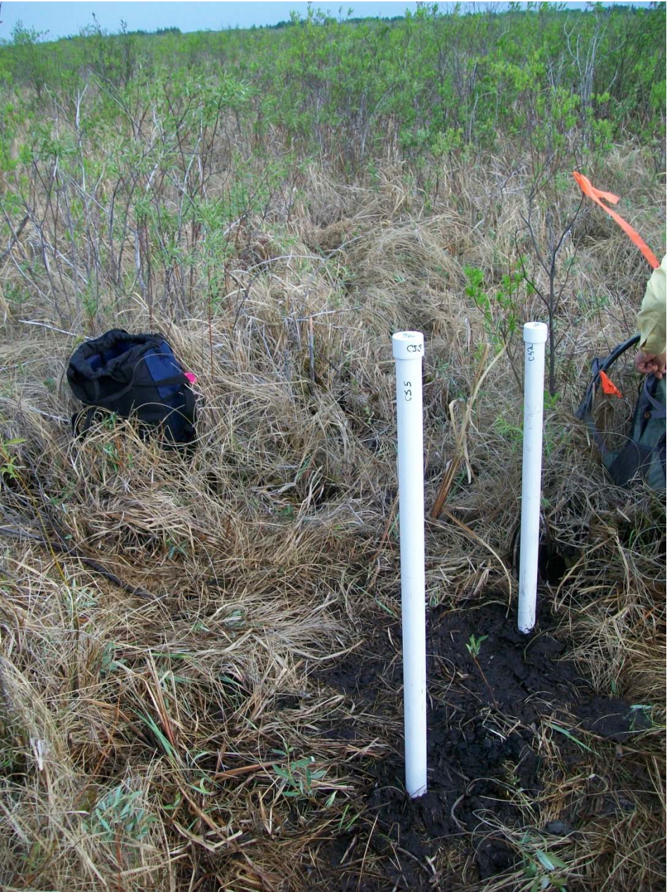
Piezometer CS2 and CS5 (deep piezometer)
