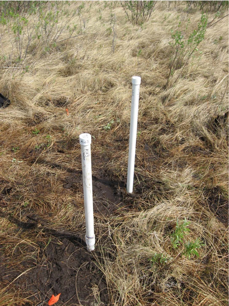
Piezometer AW3 and AW5(deep piezometer) Co-located
