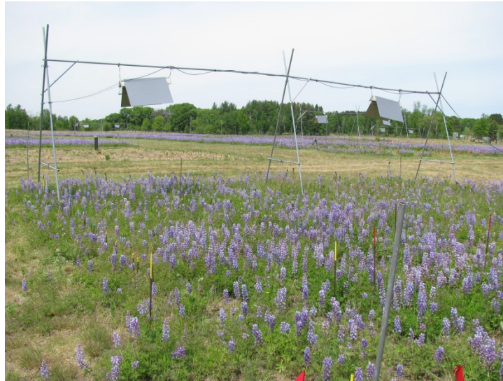
Figure 6 (above) shows the experimental set up in the field. The heat lamps are suspended by scaffolding and warm patches of prairie plants that vary in number of species (1, 4, 16, or 32 species). High warming results in \sim 2.5\text{ }^{\circ}\text{C} increase in surface soil temperature, while the low warming treatment elevates surface soil temperature by \sim 1\text{ }^{\circ}\text{C} .
