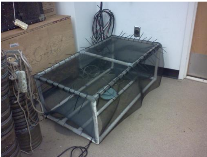
Figure 3-2 - Bioacoustic trap for round gobies
