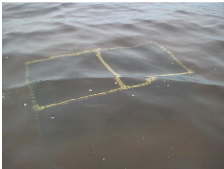
Figure 3-2 - Bioacoustic trap for round gobies deployed in Duluth Superior Harbor
