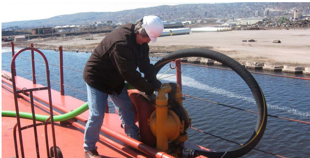
Photo 20 - Rigging transfer pump and hose on main deck
