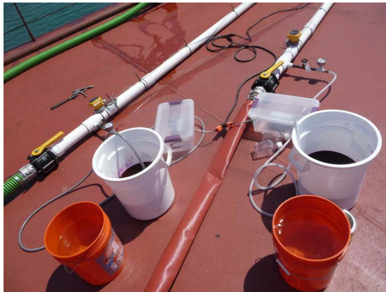
Photo 15 - Nozzle equipment on deck: hoses, valves, meters, chemical injection equipment
