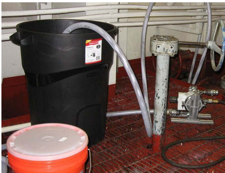
Photo 13 - Typical drum and small pump with hoses connected
