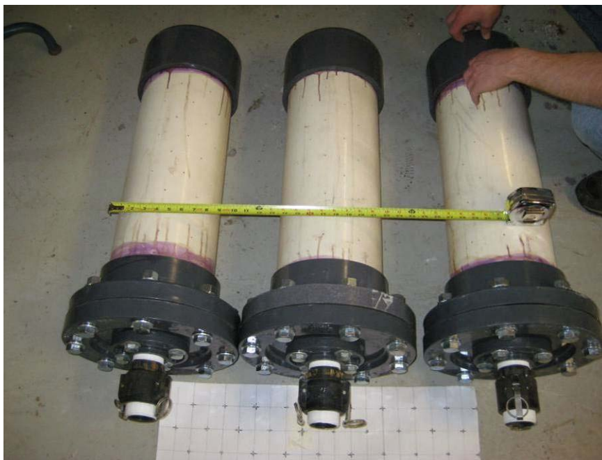
Photo 16 - Point diffusers, 10" diameter pipes 36" long with ~100 1/8" holes
