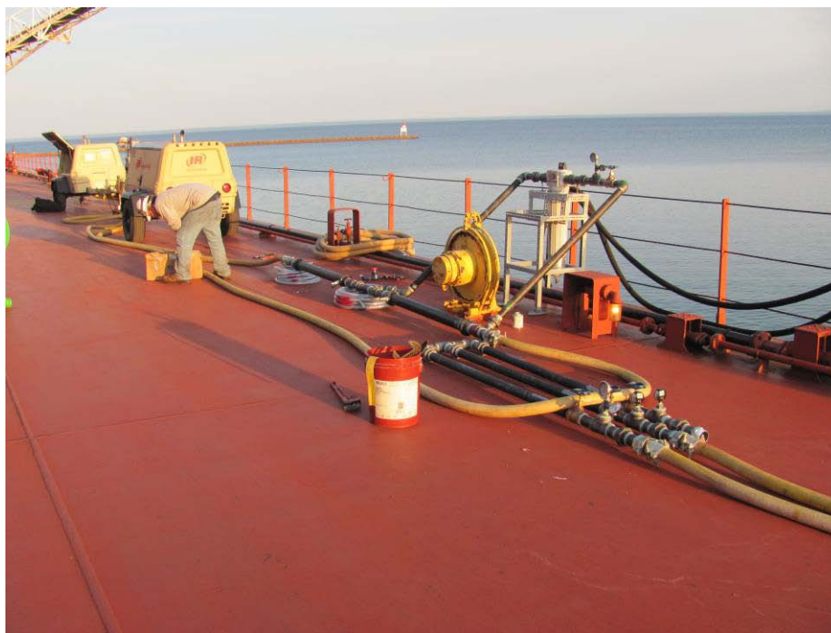
Photo 18 – Air supply equipment on deck for point diffuser and grid diffuser trials
