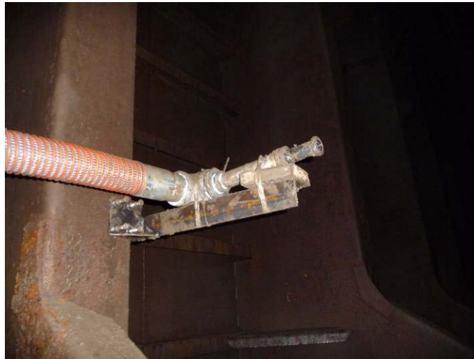
Photo 14 - Nozzle mounted to ship's structure in tank in parallel nozzle arrangement
