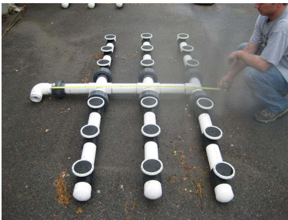
Photo 17 – Diffuser grid of 18 coarse bubble puck diffusers
