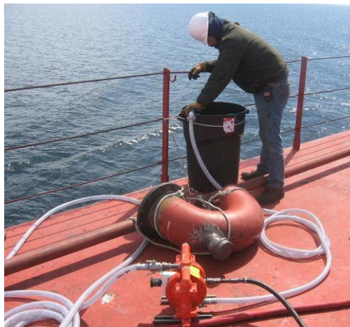
Photo 10 - Perforated hose setup on deck during dye study
