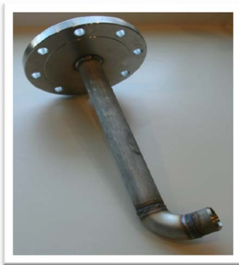
Figure 6. Sample Pitot and Sample and Return Port Flange.
