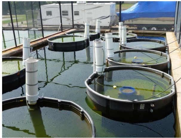
Figure 1. Example of experimental setup. Three blocks of three mesocosms were placed in outdoor enclosures. Mesocosms were equipped with biofilters and submersible pumps to aid with denitrification and circulation. Mesocosms pictured above are set up for bluegill exposures with artificial nests to promote spawning.
