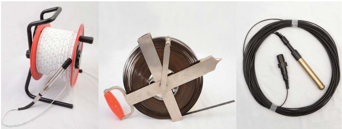
FIGURE 15. Common tools used for groundwater level monitoring (left to right): electronic tape, steel tape, data logger.
