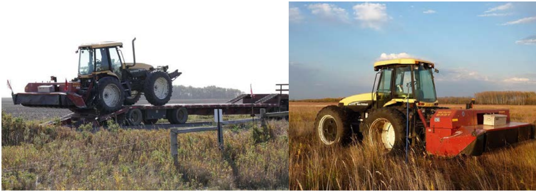
Figure 33. A disc bine cutter mounted on a four-wheel drive tractor was used during the 2010 harvest and had several advantages, including ease of loading onto a trailer.
