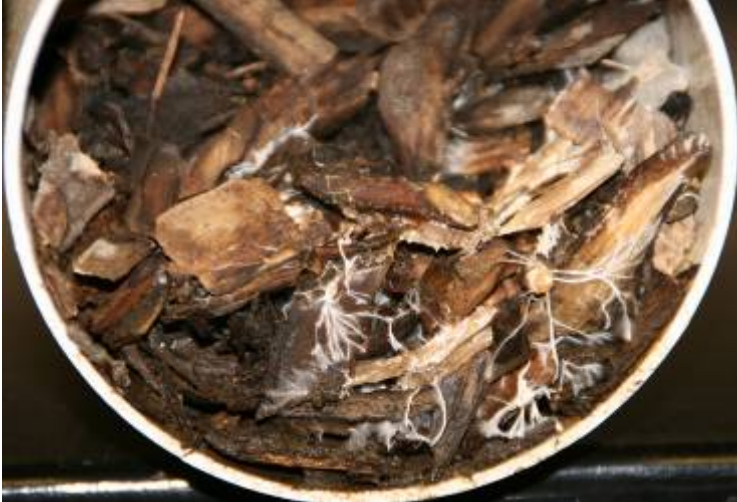
Figure 32: Fungal growth on Morris woodchips after the pulse experiment
