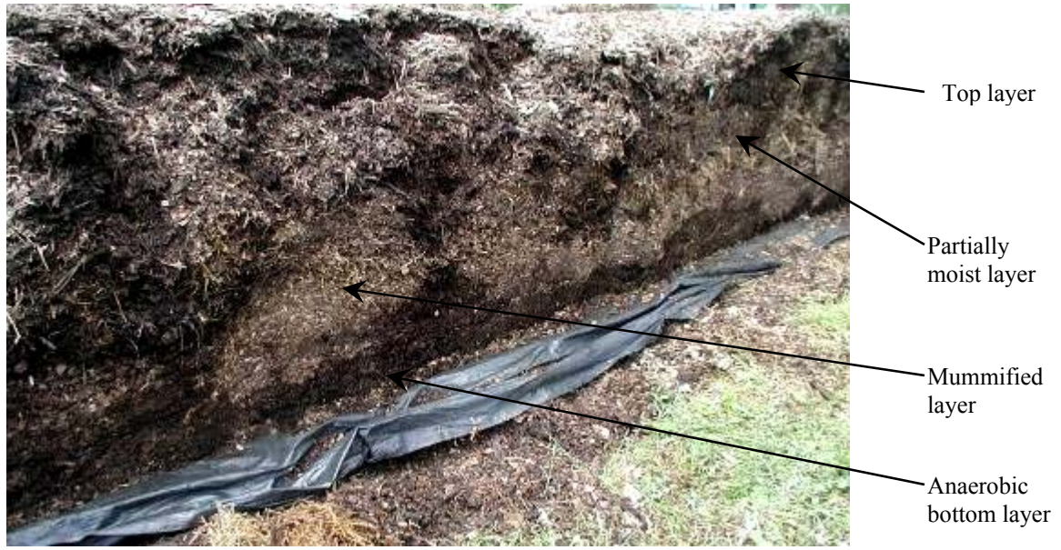
Figure 40: Layering of the biofilter after two year field study
