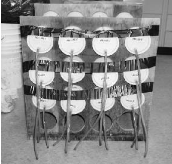
Figure 1: Front face of bioreactor tubes including drainage lid in holding rack
