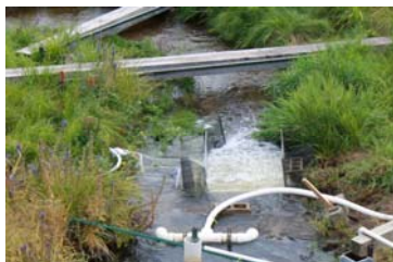
In-stream testing of a sonic and air bubble based fish barrier for deterring carp at the St. Anthony Falls Laboratory; the barrier was developed with ENRTF funding—LCCMR site visit, 09/27/11 [ML 2009: Underway]
