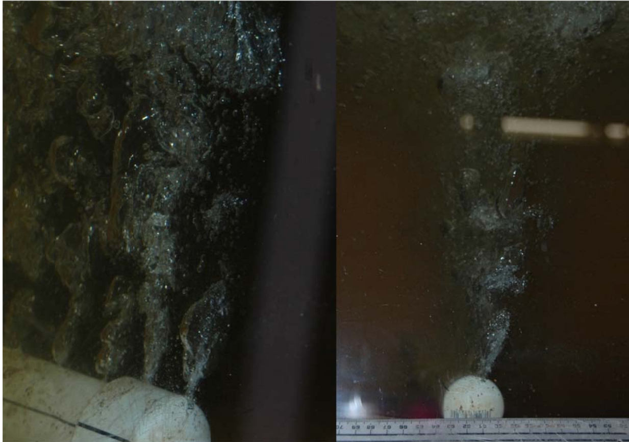
Figure 1. Typical bubble curtain provided by coarse-bubble diffuser (1mm holes at 2.5 cm spacing)
