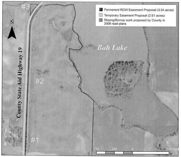
Site #1: Original design plans called for encroaching 80 feet into the easement to remove fill and slope at 7:1, thereby destroying existing grassland/brush vegetation. This encroachment has been eliminated in the 2009 plans.
